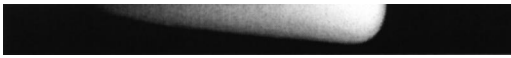
FIG. 1. Pulse of H^+ propagating to the right within the stable alkaline F state (grey scale: minimum black, maximum white). The CSTR is located at the bottom, the impermeable wall at the top. Strip width: l=0.5 mm, [OH^-]_0=1.093 \times 10^{-2} M.
